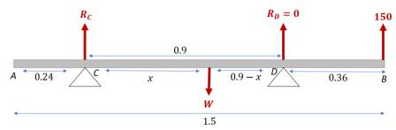
Equations with unknown distance, x, measured from C.
